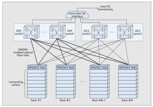
Figure 1. LIGHTNESS approach: flattened DCN architecture.
