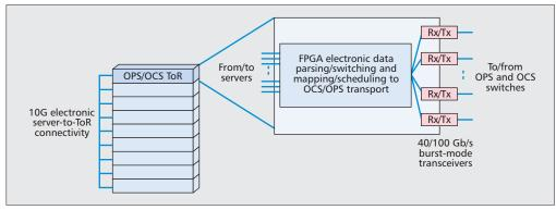
Figure 2. ToR switch architecture for the hybrid OPS/OCS DCN.
