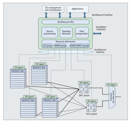
Figure 4. Unified SDN-based control plane architecture.
