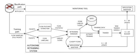
Fig. 1 Application Identifier and Autonomic Retraining System Architecture
