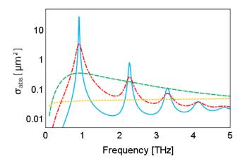
Fig. 10. Absorption cross section (in logarithmic scale) of a graphenna as a function of frequency, for different values of the relaxation time:  $10^{-14}$  s (yellow dotted line),  $10^{-13}$  s (green dashed line),  $10^{-12}$  s (red dot-dashed line) and  $10^{-11}$  s (blue solid line).
