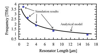
Fig. 2. Dependence of the first resonance of an infinitely wide graphenna as a function of its length. The solid line is as calculated using the analytical model and the stars correspond to the resonance frequencies obtained by simulation.
