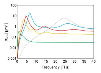
**Fig. 8.** Absorption cross section (in logarithmic scale) of a graphenna as a function of frequency, for different values of the chemical potential: 0 (green line), 0.5 (yellow line), 1 (red line) and 2 eV (blue line). The results are compared to that of an equivalent gold antenna with the same size (gray dashed line).
