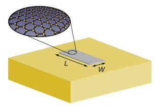
Fig. 1. Schematic diagram of a graphene-based plasmonic nano-antenna, or graphenna.
