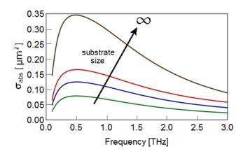
Fig. 4. Absorption cross section of a graphenna, for different substrate sizes: 6x6 μm, 10x10 μm, 16x16 μm and infinite (below to above).
