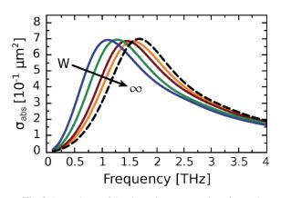
Fig. 3. Dependence of the absorption cross section of a graphenna as a function of its width. The absorption cross section normalized to the graphenna width is shown. The length of the graphenna is  $L = 5 \mu m$ . The plots correspond to infinite, 10  $\mu m$ , 5  $\mu m$ , 2  $\mu m$  and 1  $\mu m$  wide patches (right to left).
