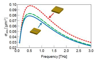
Fig. 6. Absorption cross section of a graphenna, for different positions of the graphene patch: in the center of the substrate (blue solid line), at 1.25 μm from the center (green dashed line) and at 2.5 μm from the center (red dotted line).
