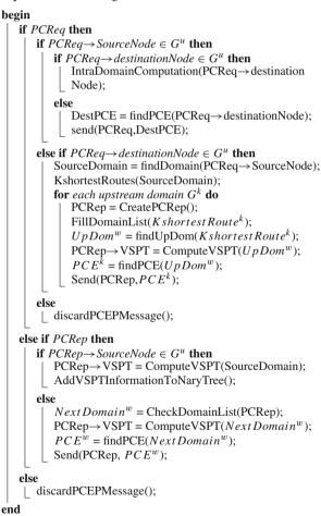
Algorithm 1: *k*-BRPC Path Computation Procedure for PCE<sub>*i*</sub>
