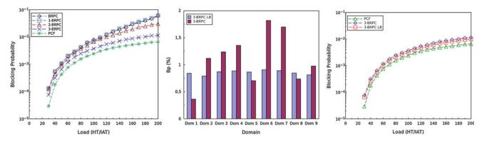
Fig. 3 Connection blocking probability: global (left); distributed among domains (center); using load balancing (right)
