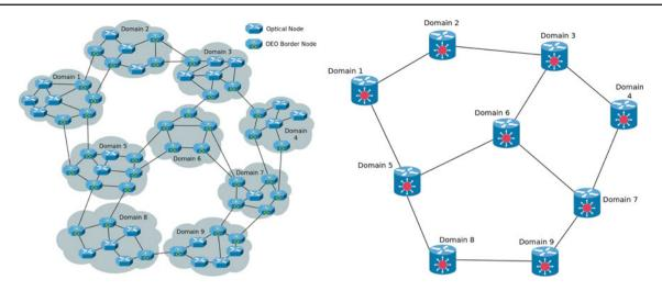
Fig. 2 Nine-domain test network topology (left). Nine-domain connectivity graph (right)
