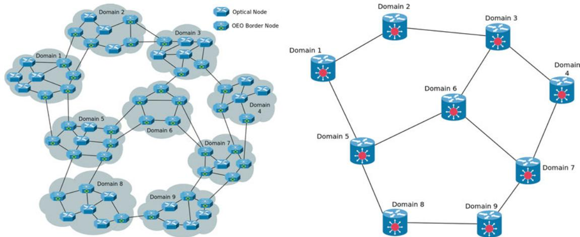
**Fig. 2** Nine-domain test network topology (left). Nine-domain connectivity graph (right)
