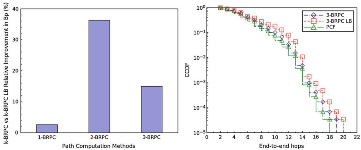
**Fig. 4** Relative blocking probability improvement between  $k$ -BRPC and  $k$ -BRPC LB path computation methods (left); CCDF of end-to-end hops for 3-BRPC, 3-BRPC LB, and PCF (right)
