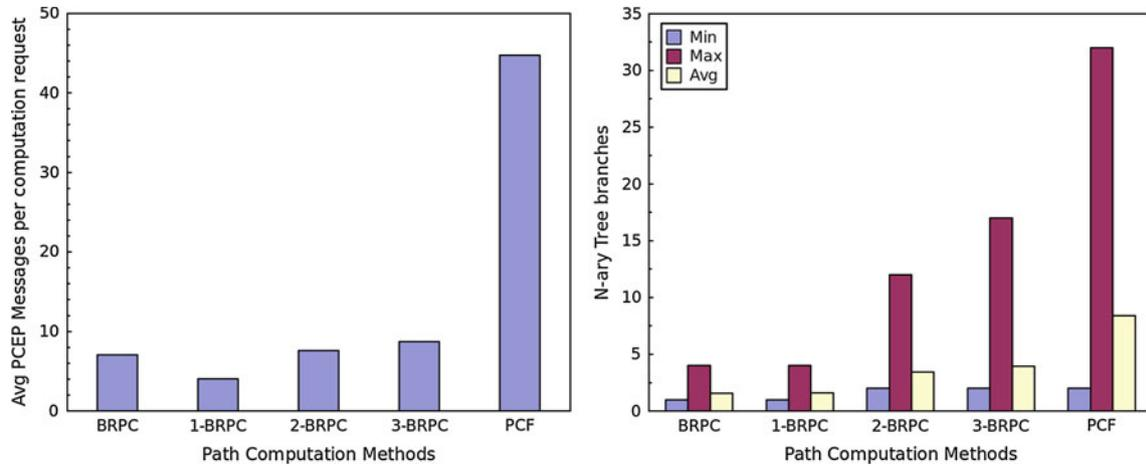
**Fig. 5** Average PCEP messages per inter-domain computation request (left); path computation complexity (right)
