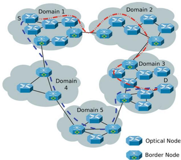
**Fig. 1** Possible end-to-end routes between S and D
