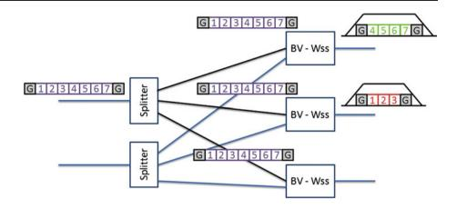
Fig. 4 Shared splitting node architecture
