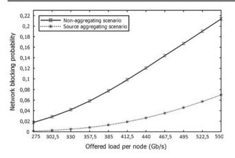
Fig. 6 Network blocking probability for different offered loads
