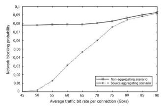
Fig. 7 Network blocking probability for different average traffic bit rates
