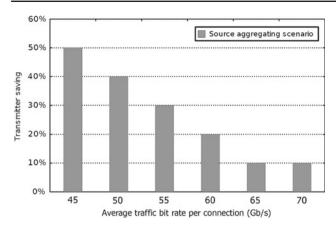
Fig. 8 Transmitter savings for different average traffic bit rates
