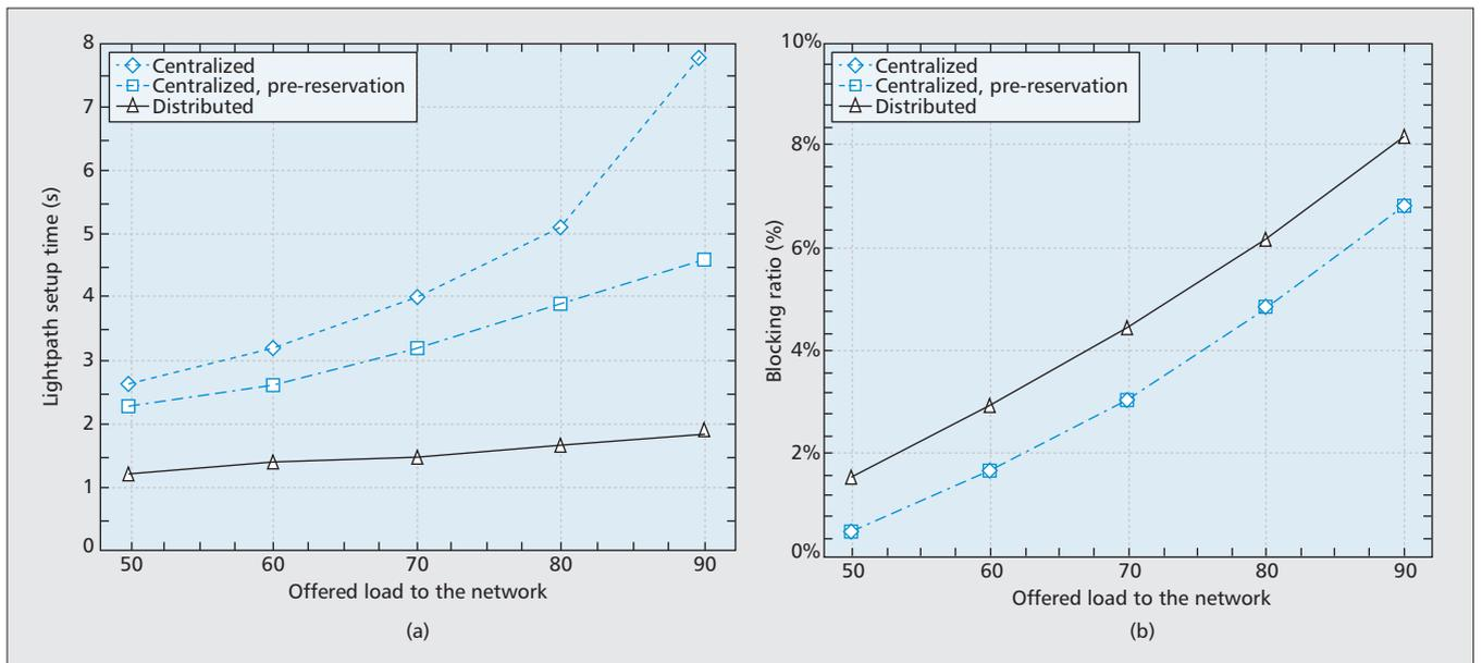
**Figure 6.** a) Measured lightpath setup time of the two schemes for an operational scenario with the traffic load varying from 50–90 Erlangs; the setup time of the centralized approach is improved using an alternative strategy (square marks, dashed line) where the wavelengths are pre-reserved to avoid waiting for the OSPF-TE flooding; b) corresponding blocking ratio results of the two schemes.
