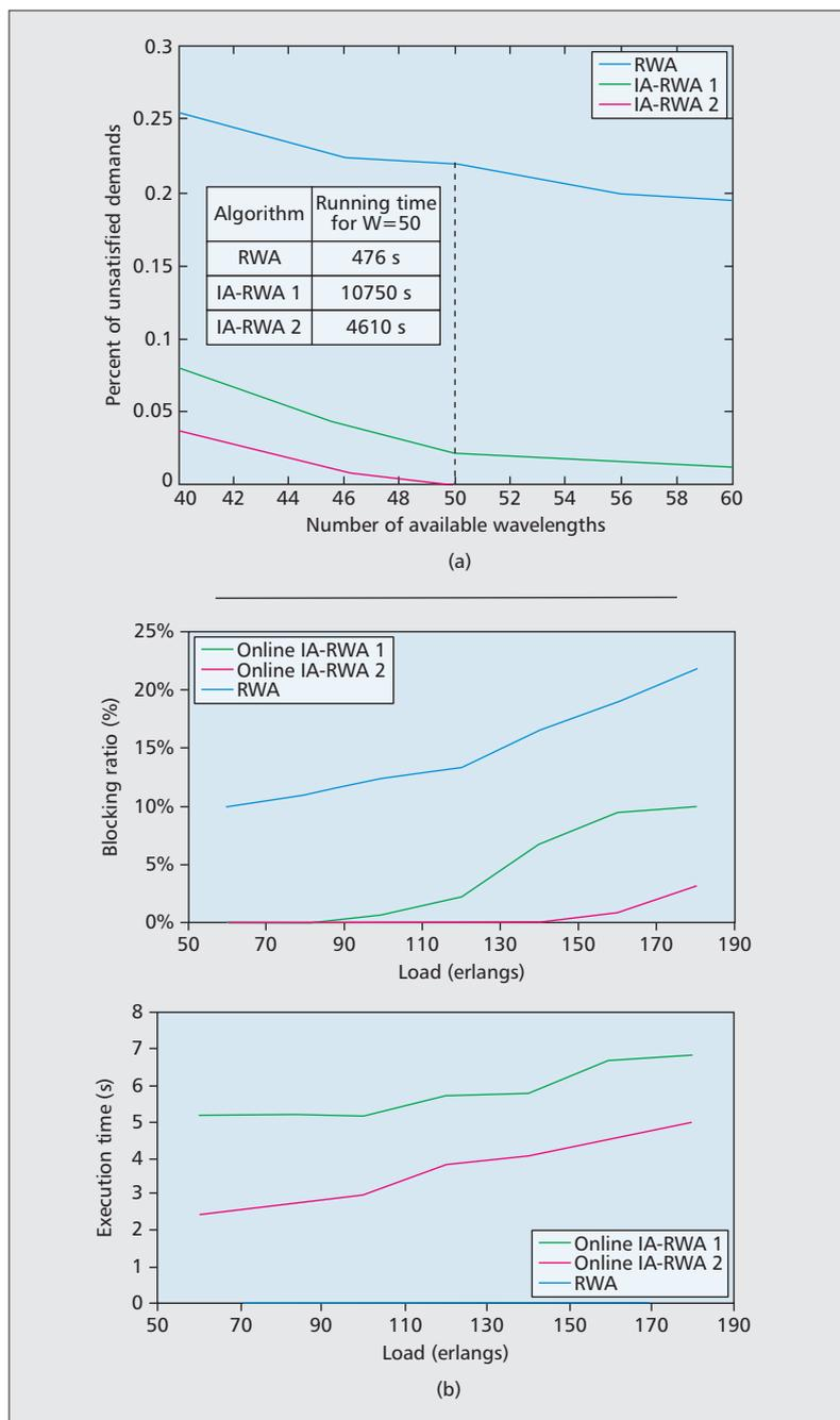
**Figure 1.** a) Offline IA-RWA blocking ratio and running times as a function of the available wavelengths  $W$ ; b) online IA-RWA blocking ratio and average execution time per connection in seconds presented as a function of the network load for a fixed number of wavelengths ( $W = 20$ ).
