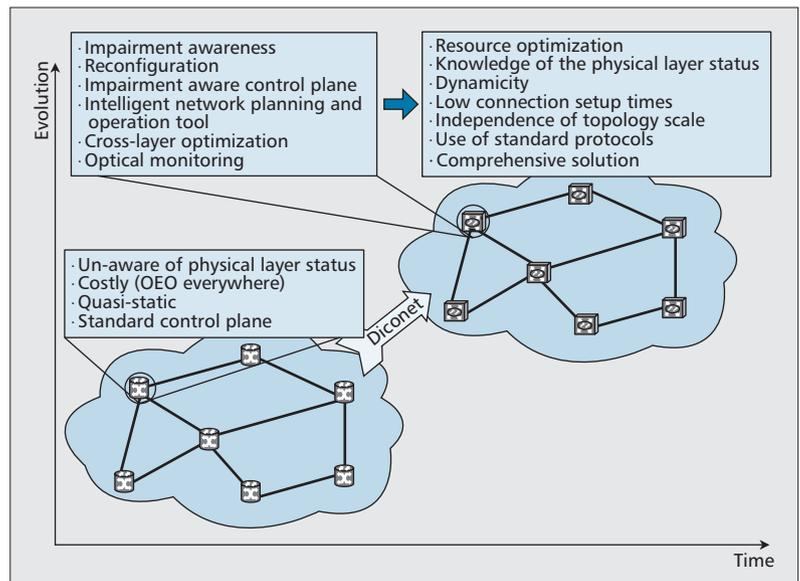
Figure 2. Current core optical networks and DICONET.
