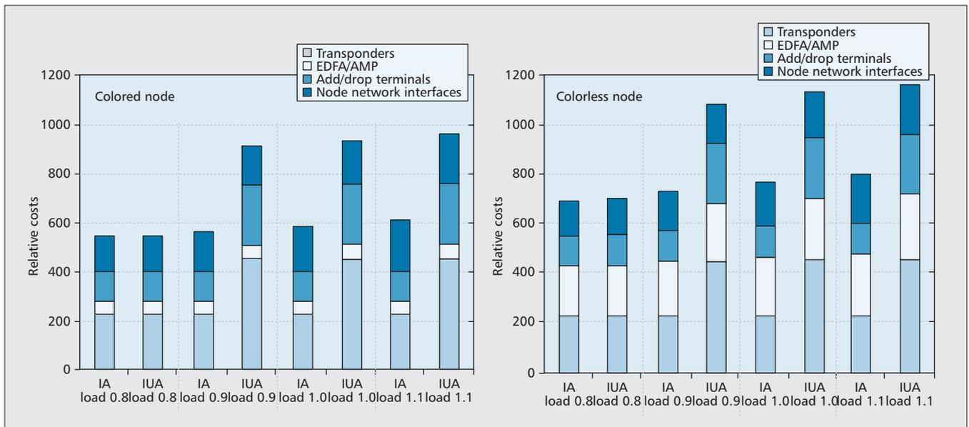
Figure 7. CapEx of IA vs. IUA for two different types of node architectures, a colored and a colorless one.
