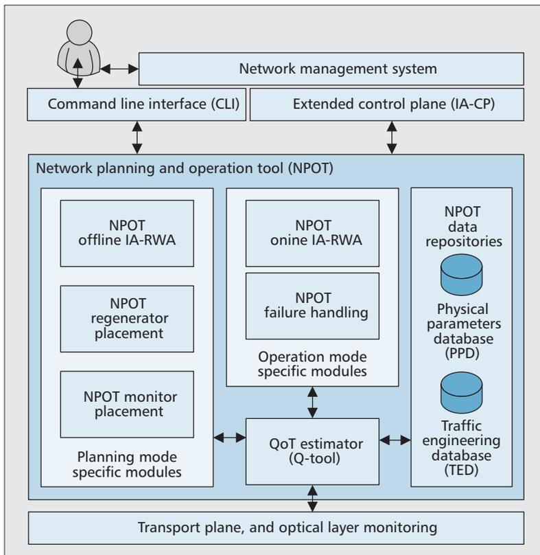
Figure 3. Anatomy of DICONET network planning and operation tool.
