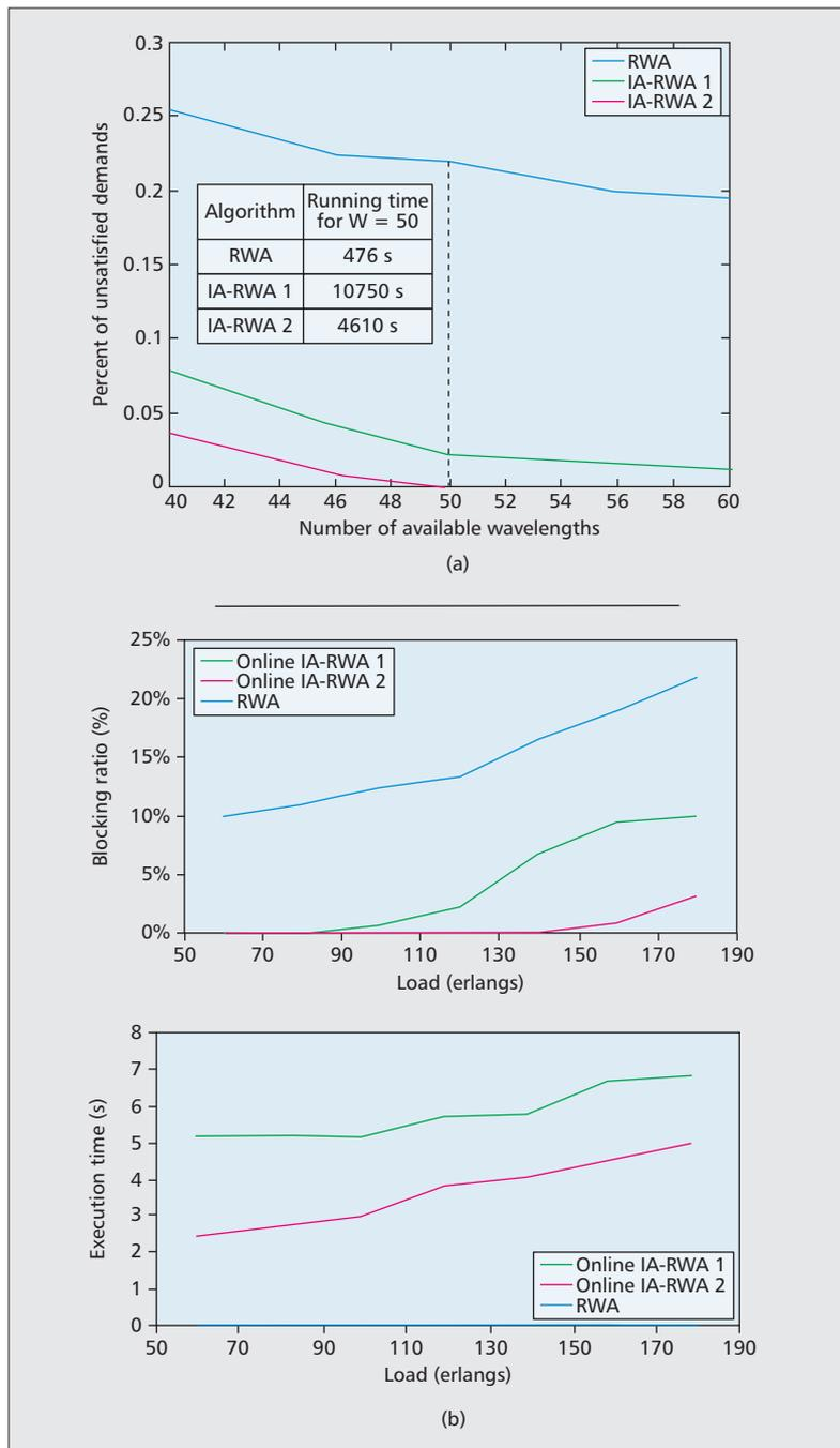
**Figure 4.** a) Offline IA-RWA blocking ratio and running times as a function of the available wavelengths  $W$ ; (b) online IA-RWA blocking ratio and average execution time per connection in seconds presented as a function of the network load, for a fixed number of wavelengths ( $W = 20$ ).
