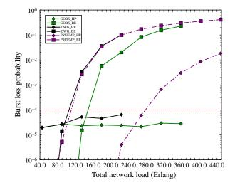
Fig. 7. (Color online) EON network: HP-BE traffic ratio of 40%-60% for the three QoS techniques: i) GOBS, ii) DWG and iii) preemption.
