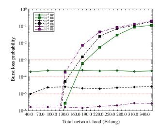
Fig. 4. (Color online) GOBS control model: validation of the LSP dimensioning model with respect to 3 different QoS demands of  $10^{-3}$ ,  $10^{-4}$ ,  $10^{-5}$  in the NSF network.
