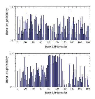
Fig. 5. (Color online) HP burst losses with uniform (top) and non-uniform (bottom) traffic in the NSF network ( $QoS = 10^{-3}$ ).
