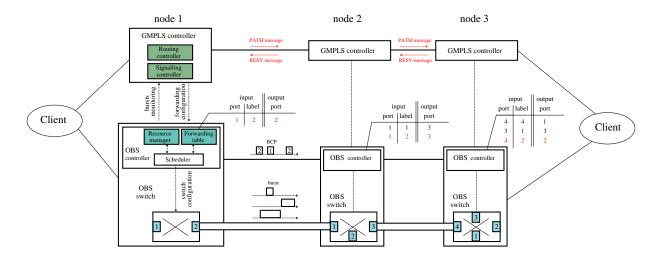
Fig. 1. (Color online) Example of a b-LSP establishment in the GMPLS/OBS network architecture.
