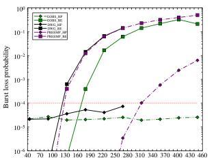
Fig. 6. (Color online) NSF network: HP-BE traffic ratio of 40%-60% for the three QoS techniques: i) GOBS, ii) DWG and iii) preemption.
