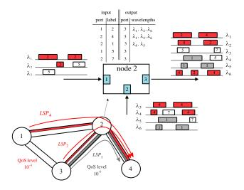
Fig. 2. (Color online) GMPLS/OBS virtual topology and the effect on the burst forwarding.
