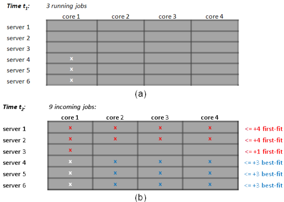
Figure 5: Visualization of first-fit and best-fit allocation strategies for a subset of 6 servers with 4 cores each. At time t_1 , there are three running jobs arranged (as result of previous allocations) as in (a); at time t_2 , nine new jobs arrive (b). First-fit will use up to 2x more servers than best-fit.
