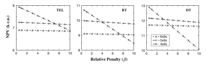
Fig. 9 NPV against  $\beta$  for medium network loads (i = 3) in TEL (*left*), BT (*center*), and DT (*right*) networks
