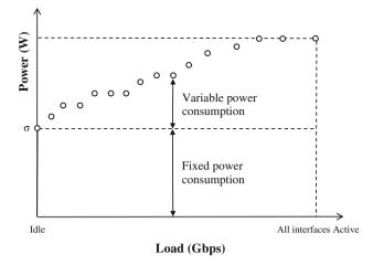
Fig. 2 Model of IP/MPLS node power consumption as a function of the load
