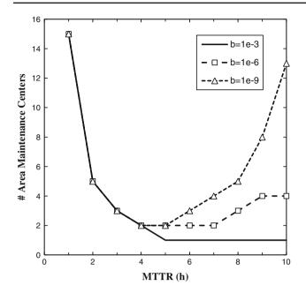
Fig. 7 Number of area maintenance centers to open as a function of the MTTR objective
