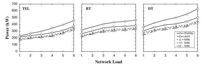
Fig. 6 Power consumption of the considered approaches as a function of the network load in TEL (left), BT (center), and DT (right) networks
