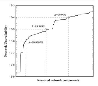
Fig. 1 Network unavailability evolution versus removed network components
