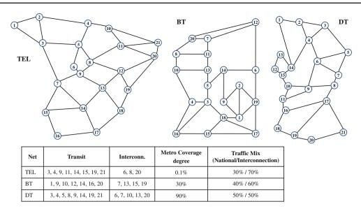
Fig. 4 Sample optical network topologies used in our tests: 21-node Spanish Telefónica (*left*), 20-node British Telecom (*center*), and 21-node Deutsche Telecom (*right*). A table with details of the IP/MPLS topologies as well as the IP/MPLS traffic mix is also provided
