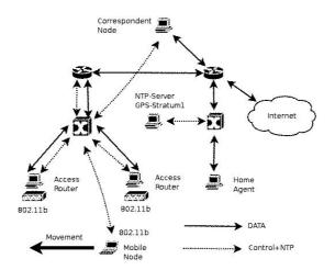
Fig. 1. Measurement scenario simplified structure
