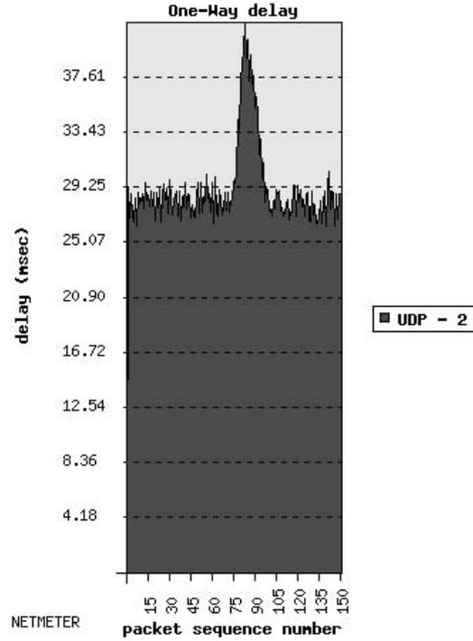
Fig. 3. OOO packet burst effects on one-way delay
