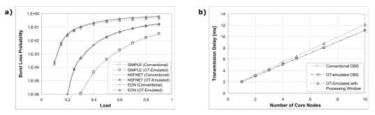
Figure 4. Comparison of the performance, a) Burst Loss Probabilities and b) Transmission Delays.
