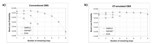
Figure 3. Burst loss probability vs. remaining hops number, in A) conventional and B) OT-emulated OBS.
