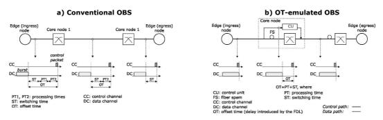
Figure 1. OBS architectures, a) conventional and b) OT-emulated.
