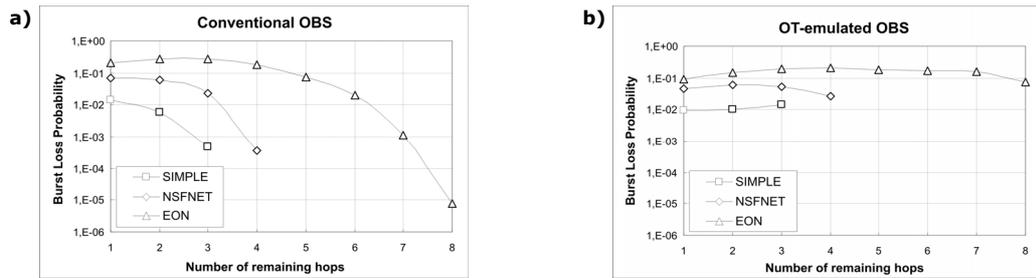
Figure 3. Burst loss probability vs. remaining hops number, in A) conventional and B) OT-emulated OBS.
