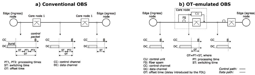
Figure 1. OBS architectures, a) conventional and b) OT-emulated.
