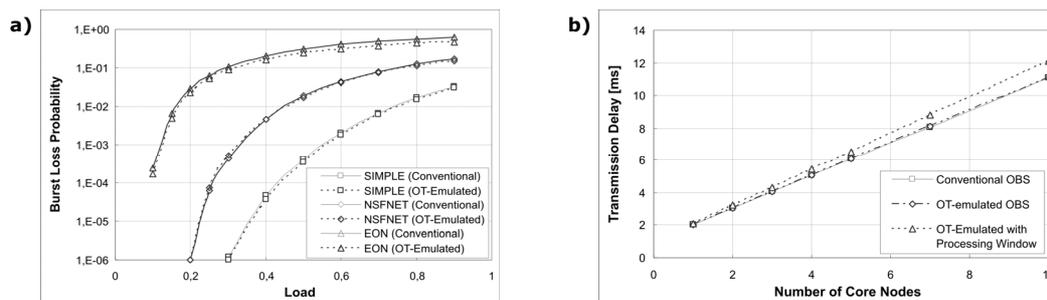
Figure 4. Comparison of the performance, a) Burst Loss Probabilities and b) Transmission Delays.
