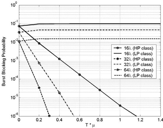
Fig. 6. Burst Blocking Probability as a function of the preemption window normalized by the mean burst duration and of the number of wavelengths ( $\alpha = 25\%$ ,  $\rho = 0.8$ )
