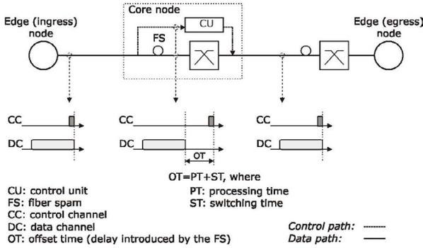
Fig. 1. OBS architecture for burst preemption mechanism
