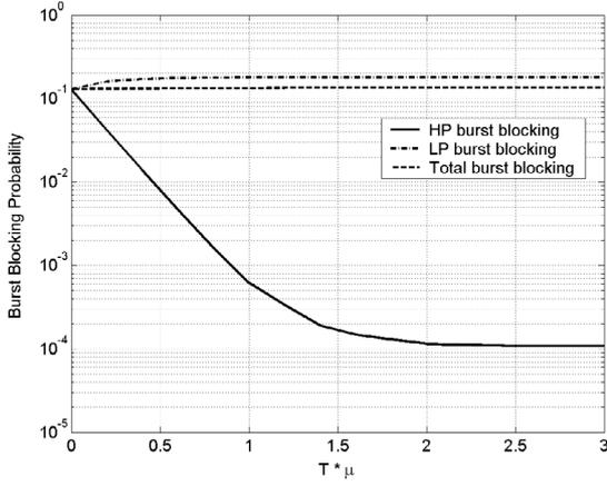
Fig. 5. Burst Blocking Probability as a function of the preemption window normalized by the mean burst duration
