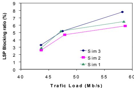
Fig. 6. LSP Blocking Ratio due the impossibility of finding a LSP with the required Bw in the ND3
