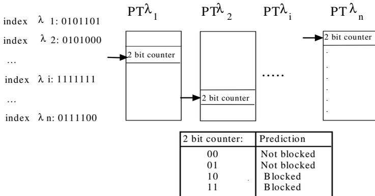
Fig. 1. Example of Prediction Table access and values of the 2-bit counters
