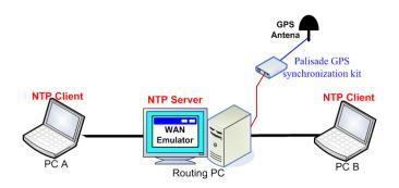
Figure 6. Testbed with Synchronization Kit
