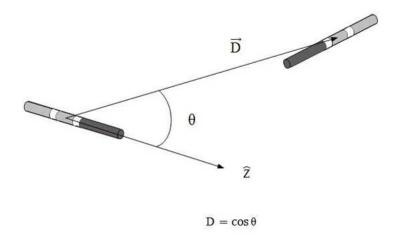
Figure 4: Directionality of the catalytic nanomotor
