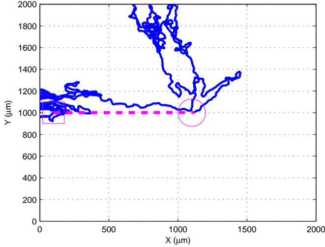
Figure 5: Trace of the catalytic nanomotor from the transmitter (square) to the receiver (circle)
