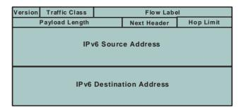
Figure 1: The IPv6 Header Format.
