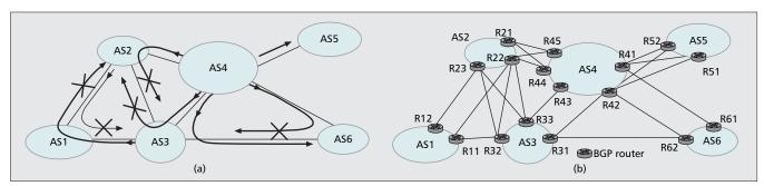
**Figure 1.** *a)* The export policies and the power-law relationship of the Internet topology make AS-graphs inadequate to find disjoint paths across domains; b) the same topology but at a border router level.
