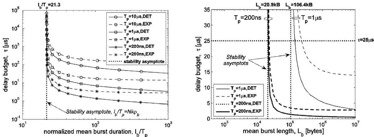
Figure 2. Delay budget vs.: A) normalized mean burst duration, B) mean burst length.
