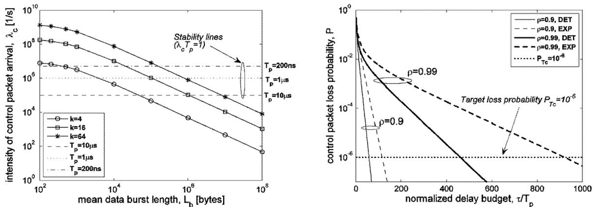
Figure 1. A) Intensity of control packet arrival; B) Loss probability of control packets.
