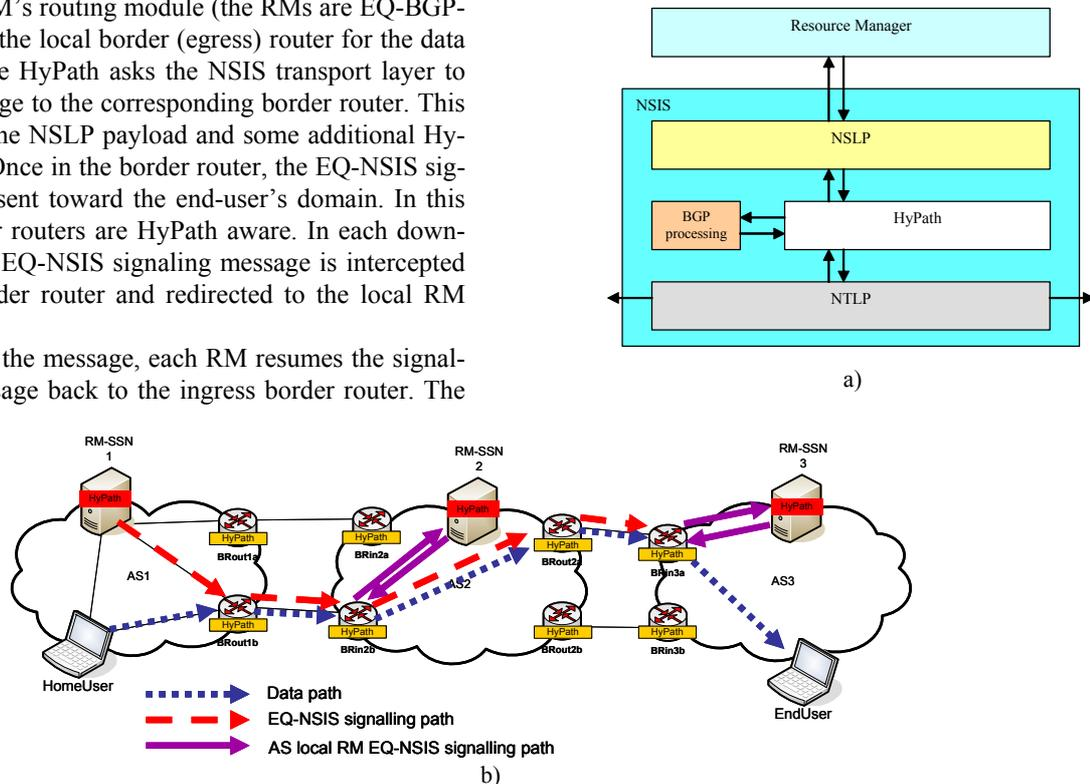
Fig. 4. NSIS architecture: a) HyPath in the EQ-NSIS architecture; b) EQ-NSIS signaling with HyPath.
