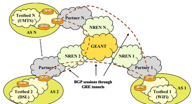
Fig. 1. Access networks, NRENs and GEANT architecture.
