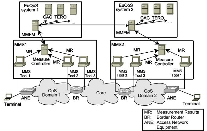
Fig.5. The Monitoring and Measurement System (MMS).
