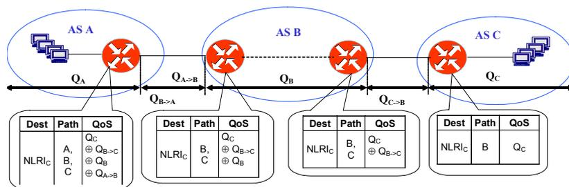
Fig.6. Example of EQ-BGP operation.
