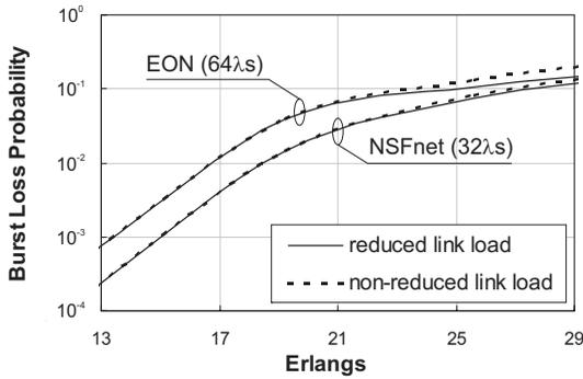
Fig. 2. Accuracy of non-reduced link load model.
