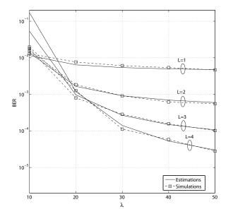
Fig. 8 BER values versus the number of samples per chip  $\lambda$  in the case of K = 1,  $\beta = 64$ ,  $E_b/N_0 = 6dB$  with the increment of L
