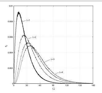
Fig. 4 Probability mass function (PMF) of the variable C in the case of  $\beta = 64, \lambda = 30, E_b/N_0 = 10 dB$  with the increment of the number of secondary paths L.
