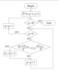
Fig. 3 Algorithm for the calculation of N elements in the vector  ${f E}$
