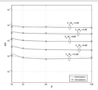
Fig. 7 BER values versus the spreading factor  $\beta$  in the case of  $K=1,\,L=2,\,\lambda=30$  with the increment of  $E_b/N_0$
