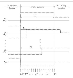
Fig. 2 Illustration of the signal components at the output of the channel and their sampling process in the receiver
