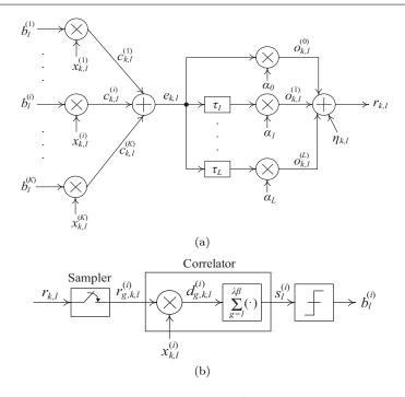
**Fig. 1** Block diagram of the chaos-based DS-CDMA communication system under study: (a) The transmitting side with multiple-access operation and the generalized frequency non-selective fading channel, (b) The proposed direct-oversampling correlator-type receiver
