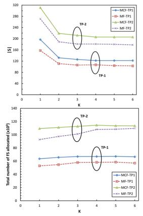
Fig. 9. Number of FSs used (top) and total number of FSs allocated (bottom) in the MCF/MF-enabled EON network with 19 cores/fibers for different values of  $K \in \{1,..,6\}$ .
