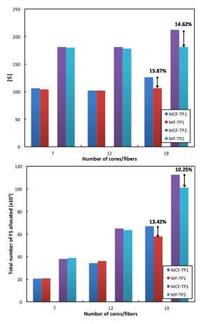
Fig. 5. Number of FSs used (top) and total number of FSs allocated (bottom) in a MCF/MF-enabled EON network with 7, 12 and 19 cores/fibers.
