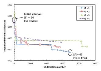
Fig. 4. Total number of FSs allocated in the 6-node TEST network along the SA iterations. The initial and final |S| values are shown.
