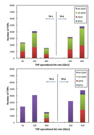
Fig. 8. Number of TXPs used at 40, 100 and 400 Gb/s in the DT with 19-core MCFs (top) and 19 fibers per MF link (bottom). Scenarios with demands following TP-1 and TP-2 are shown.
