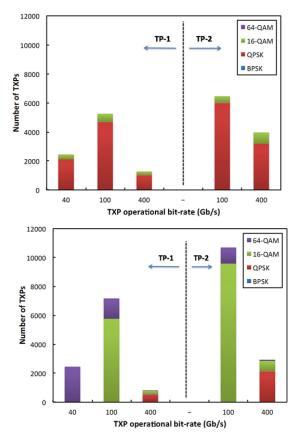
Fig. 7. Number of TXPs used at 40, 100 and 400 Gb/s in the EON with 19-core MCFs (top) and 19 fibers per MF link (bottom). Scenarios with demands following TP-1 and TP-2 are shown.
