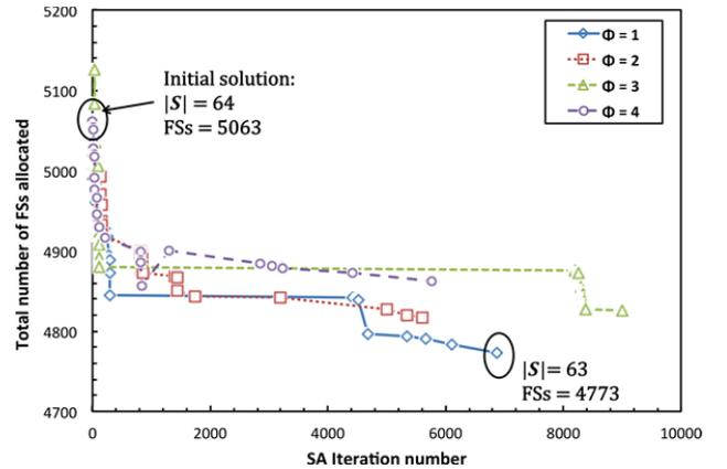
Fig. 4. Total number of FSs allocated in the 6-node TEST network along the SA iterations. The initial and final  $|\mathcal{S}|$  values are shown.
