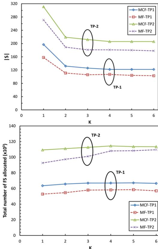
Fig. 9. Number of FSs used (top) and total number of FSs allocated (bottom) in the MCF/MF-enabled EON network with 19 cores/fibers for different values of  $K \in \{1, \dots, 6\}$ .
