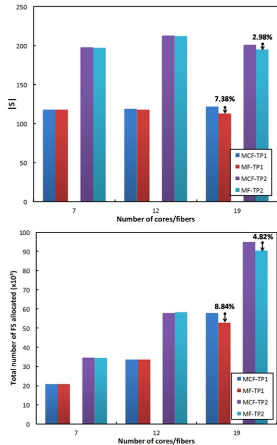
Fig. 6. Number of FSs used (top) and total number of FSs allocated (bottom) in a MCF/MF-enabled DT network with 7, 12 and 19 cores/fibers.
