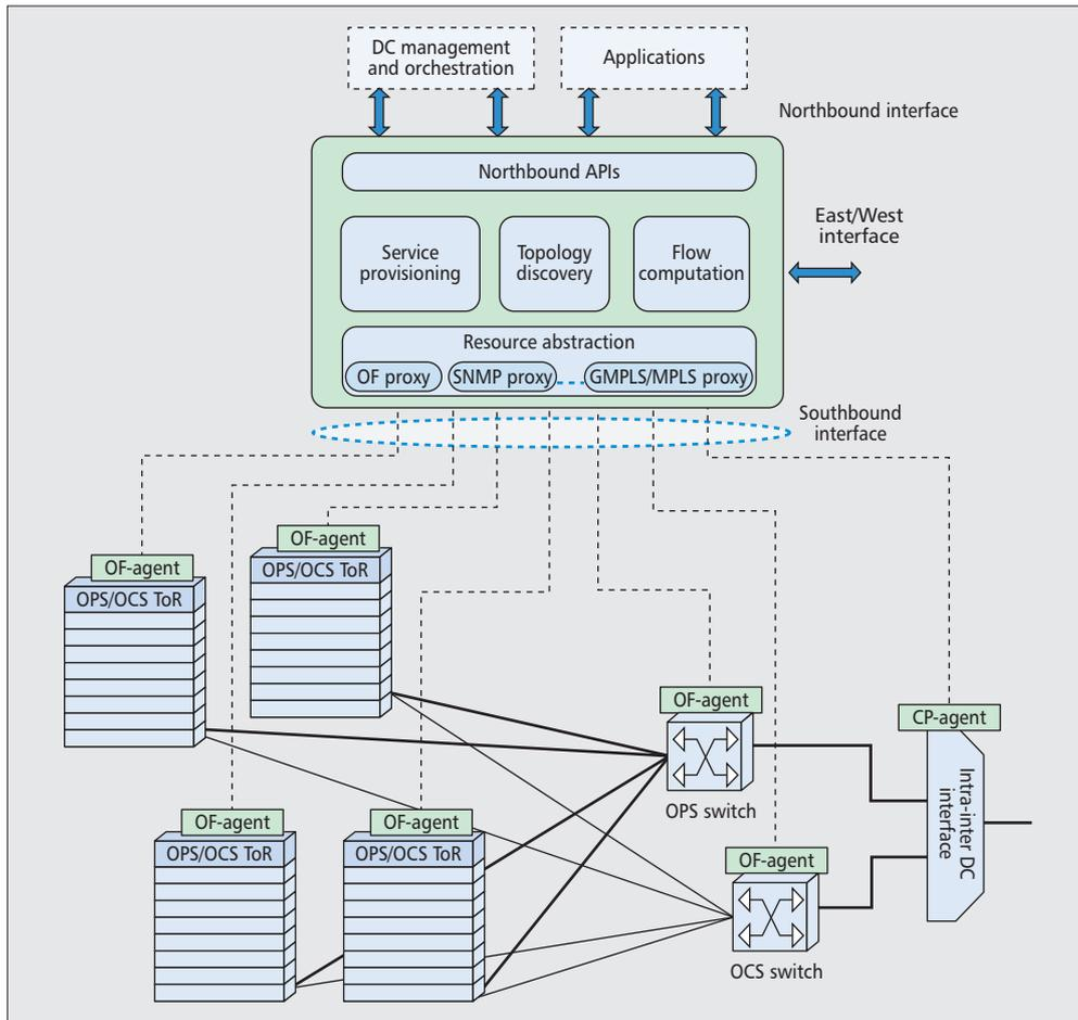
Figure 4. Unified SDN-based control plane architecture.
