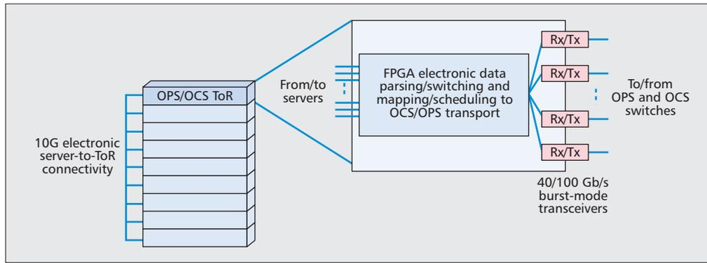
Figure 2. ToR switch architecture for the hybrid OPS/OCS DCN.
