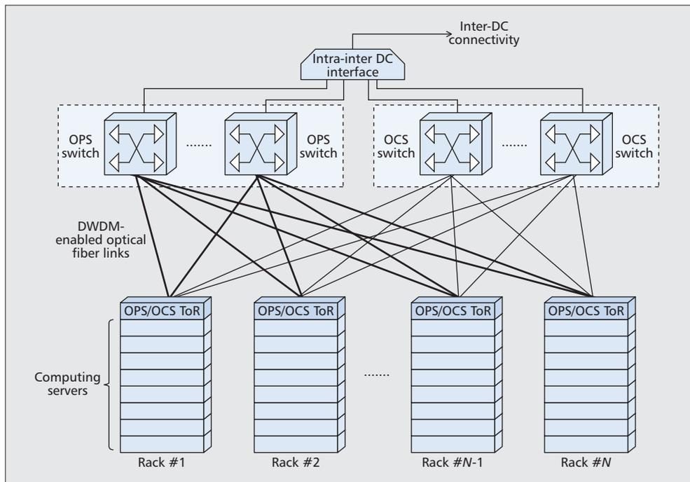
Figure 1. *LIGHTNESS* approach: flattened DCN architecture.
