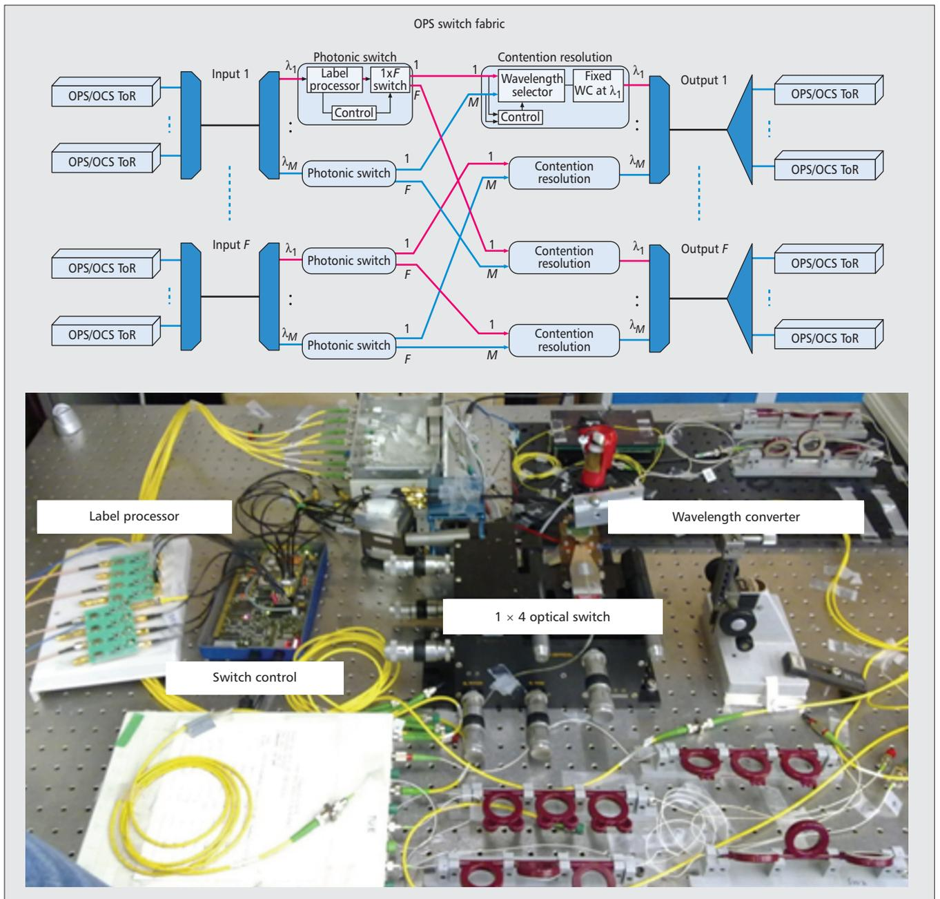
Figure 3. OPS switch: architecture described as a block diagram (top); picture of an  $F = 1$   $M = 4$  OPS switch laboratory prototype built using discrete optical components (bottom).
