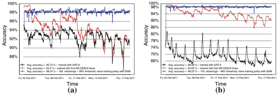
**Fig. 4** Comparative of the *Autonomic Retraining System* with other solutions. **a** Comparative without sampling. **b** Comparative with 1/1,000 sampling rate
