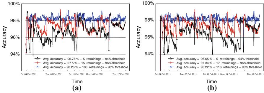
**Fig. 3** Impact of the *Autonomic Retraining System* on the *Application Identifier* with the selected configuration (i.e., naive training policy with 500K). **a** Retraining without sampling. **b** Retraining with 1/1,000 sampling rate
