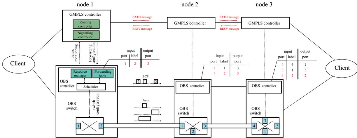
Fig. 1. (Color online) Example of a b-LSP establishment in the GMPLS/OBS network architecture.
