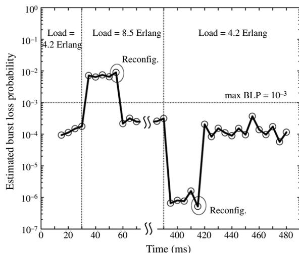
Fig. 9. Time sample showing a GMPLS-driven b-LSP reconfiguration when a traffic peak is detected and the return to the original b-LSP configuration after its decrement.
