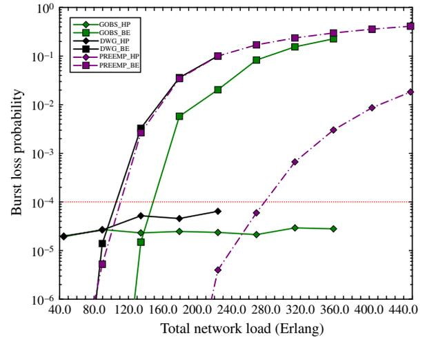
Fig. 7. (Color online) EON network: HP-BE traffic ratio of 40%–60% for the three QoS techniques: i) GOBS, ii) DWG and iii) preemption.
