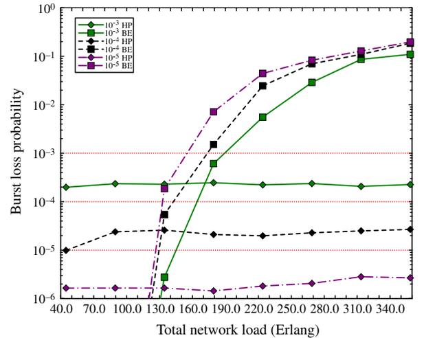
Fig. 4. (Color online) GOBS control model: validation of the LSP dimensioning model with respect to 3 different QoS demands of  $10^{-3}$ ,  $10^{-4}$ ,  $10^{-5}$  in the NSF network.
