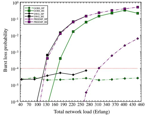
Fig. 6. (Color online) NSF network: HP-BE traffic ratio of 40%–60% for the three QoS techniques: i) GOBS, ii) DWG and iii) preemption.
