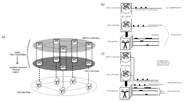
Also, allow the coexistence of WCS and OBS due to using the same GMPLS controlled network. Other advantage is the fault's isolation provision. However its importance is dependent of the signalling scheme. Possible drawbacks are the maintenance of two separate networks.
