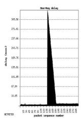
Fig. 2. FMIPv6 handover, instantaneous OWD (VoIP Traffic)
