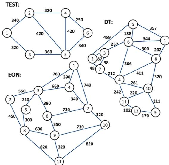
Fig. 3. Network topologies used. Link distances are shown in km.
