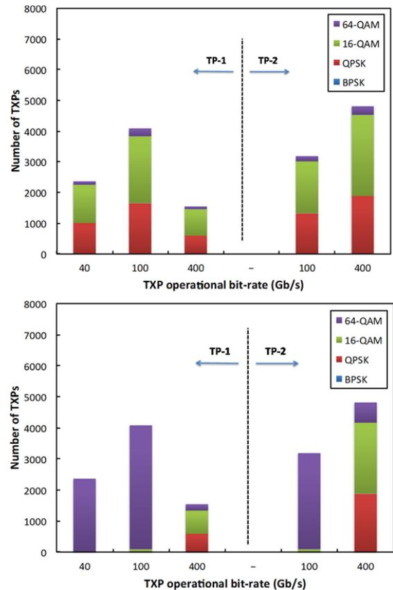
Fig. 8. Number of TXPs used at 40, 100 and 400 Gb/s in the DT with 19-core MCFs (top) and 19 fibers per MF link (bottom). Scenarios with demands following TP-1 and TP-2 are shown.
